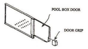
To adjust the Pool Door Grip place the set screws in either the inner or outer set of holes depending on strap size and then push Pool Door Grip in the direction shown in the illustration below.
