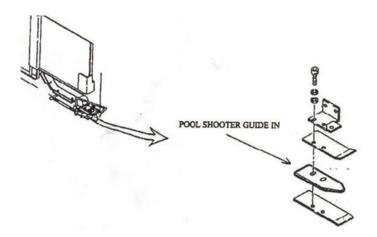
To adjust it, flip and position the Adjuster Plate and set as shown in the illustration below.
